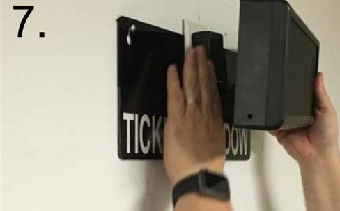
Plug the power adapter into the back of the LED Display. Then plug the power adapter into the wall outlet. Hang the LED Display on the two screws and hide any extra power cord behind the display.
